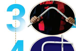
Turn the pipe bend in the direction opposite to the initial bend at the desired angle Note: The bend should be returned slowly so that no wrinkles can be seen at the bend point
