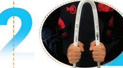
Bend the tube slowly with uniform pressure in such a way that the upper tissue of the tube is fully opened and the two sides of the tube meet each other
