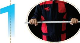
The spring should be directed into the pipe and where the desired bend should be
