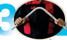
Bring the bend of the pipe at a direction opposite the initial bending back to the initial position.
