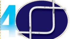
Pull the spring out of the pipe and the desired curve is ready.
