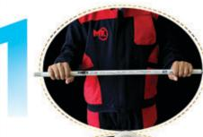
The spring must be led inside the pipe where the desired bend is to be done.
