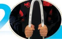
The tube should be bent slowly and with a constant pressure so that the pipe's upper tissue is completely opened and the two sides of the pipe are close
