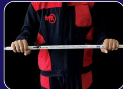
2-The tube should be bent slowly and with a constant pressure so that the pipe's upper tissue is completely opened and the two sides of the pipe are close
