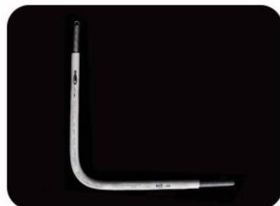
4-Pull the spring out of the pipe and the desired curve is ready.
